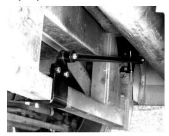
For installation of the front <u>Straight</u> TIGER TRAK stabilizer bar follow instructions 1-11. Depending on the year and model of coach as to whether you install the bar in front of or behind the front axle. (See above Photo).
